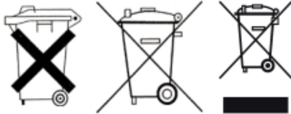
Symbols for labeling electronic devices
