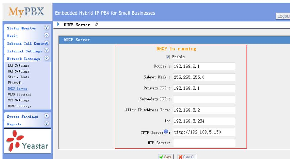
The screenshot shows the MyPBX web interface for 'Embedded Hybrid IP-PBX for Small Businesses'. The 'DHCP Server' configuration page is displayed, with a red box highlighting the 'Enable' checkbox and its associated fields. The configuration includes:
