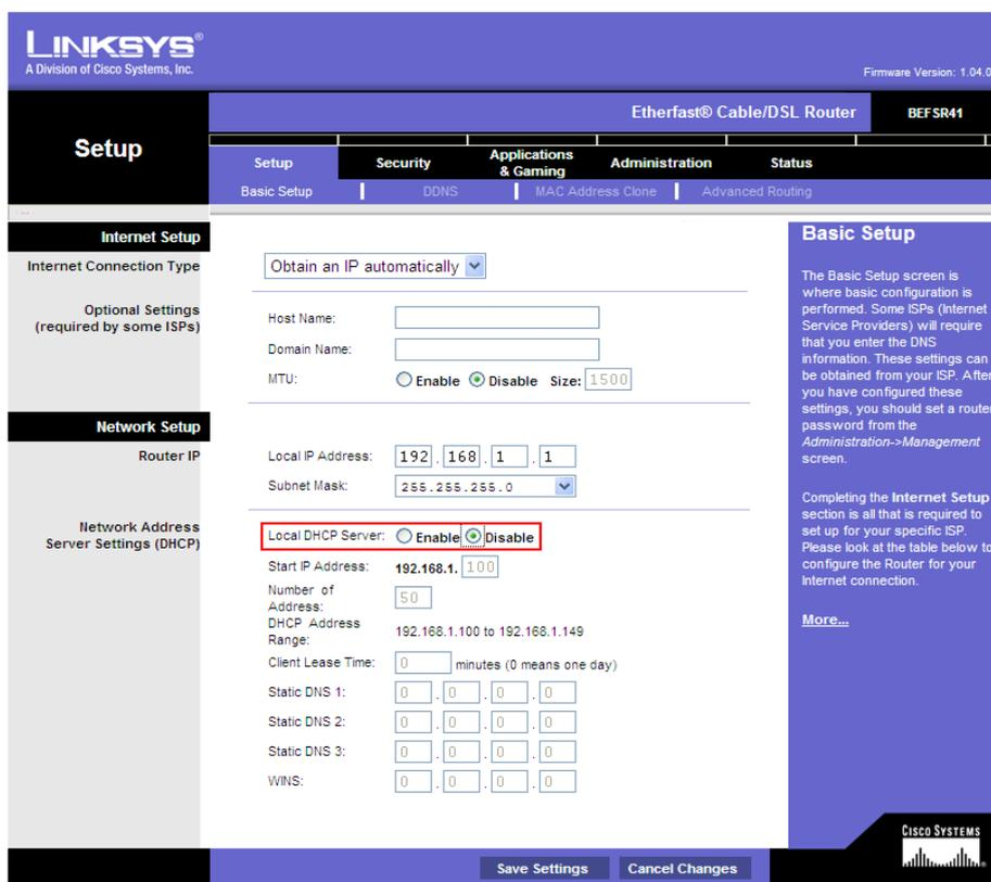
The screenshot shows the Linksys configuration interface for an Etherfast Cable/DSL Router (BEFSR41). The 'Local DHCP Server' section is highlighted with a red box, showing the 'Disable' radio button selected. Other visible settings include:
