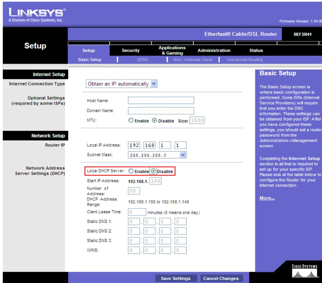
The screenshot shows the Linksys Basic Setup page for an Etherfast Cable/DSL Router (BEFSR41). The page is divided into several sections: Internet Setup, Network Setup, and Basic Setup. The Local DHCP Server settings are highlighted with a red box, showing the 'Disable' radio button selected.
