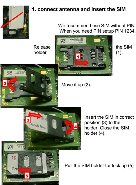
Note: All programmed parametres are saved on the SIM. The SIM you can insert into GDI already preprogrammed or setup GDI after switching ON (via bellow).
