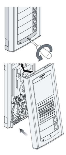
**CAUTION!** During assembly of the front panel may be needed to connect/disconnect the speaker connector (see schematics)
