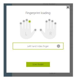
5) Place the selected finger on a external USB reader. This process is repeated three times for greater precision.
