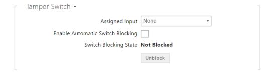
The tamper switch equipped models help detect opening of the device cover and signal this event as **TamperSwitchActivated**. The events are written into a log and read out via HTTP API (refer to the **2N** <sup>®</sup> **Helios IP HTTP API** manual).
