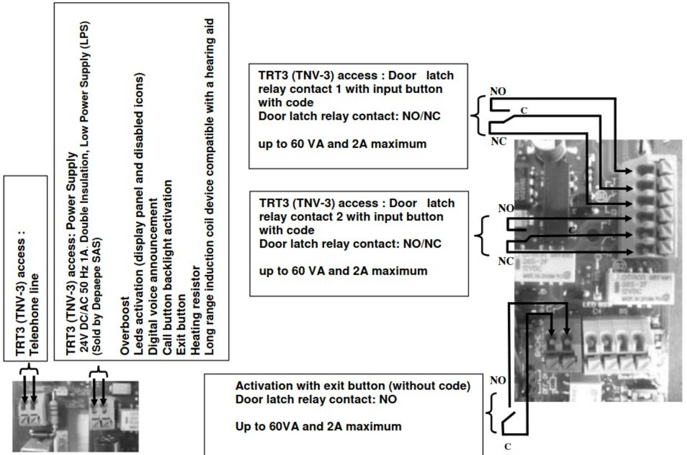
Those ports are designed to be connected on a TRT3 (TNV-3) network in accordance with EN 60950-1 : 2006 specifications.
