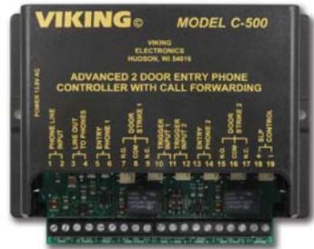
The **C-500** allows up to 6 permanent keyless entry codes plus 2 "one time use" entry codes for each door. The **C-500** provides optional entry phone distinctive ring, two trigger inputs for "Request to Exit" and field programmable Caller ID or beep tones when answered to indicate which door is activated.
