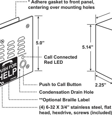
The black plastic rough-in box (part # 259576) may be purchased separately (Example: Mounting boxes to studs before the walls are finished for flush installation). Go to [www.vikingelectronics.com](http://www.vikingelectronics.com) and click on "Spare Parts" to order these rough-in boxes.
