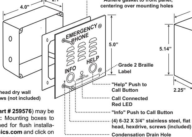
The black plastic rough-in box (part # 259576) may be purchased separately (Example: Mounting boxes to studs before the walls are finished for flush installation). Go to [www.vikingelectronics.com](http://www.vikingelectronics.com) and click on "Spare Parts" to order these rough-in boxes.
