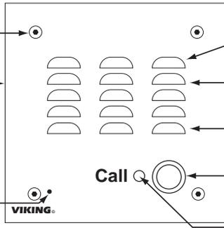
**Microphone:** Omni-directional microphone with protective water-resistant cloth.
