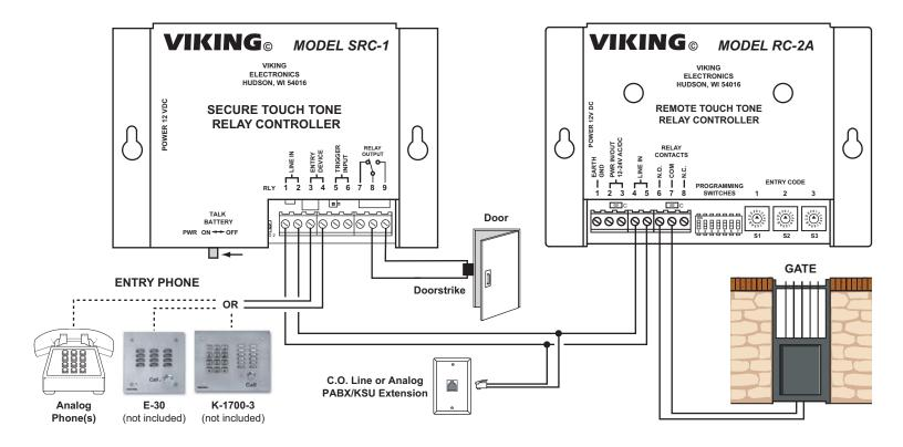
The SRC-1 provides secure relay control of a single door or gate, meaning the person at the entry phone is not able to operate it. Add an RC-2A to provide a second secure relay to operate a second door or gate.
