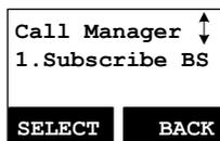
3. Press **UP** or **DOWN** key to select the desired base (#1~4), press **CHANGE** (Left) soft key to set the Subscribe BS ON/OFF.
