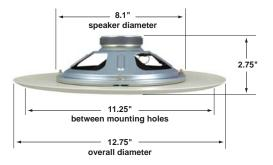
Installation: Mounting hardware for the 30AE and 35AE ceiling speakers is included for easy installation in drop ceilings or speaker enclosures. Flush mount into an 8.25" to 10.0" diameter hole.
