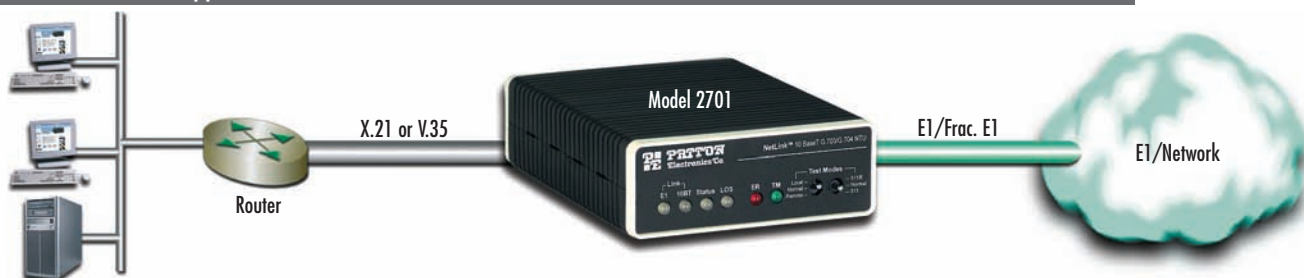
Models 2701 & 2701RC application: E1 network termination on X.21 or V.35 for data
