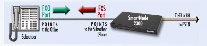
2) Connect the FXO ports on your PBX to the SmartNode's IC-4FXS card.
