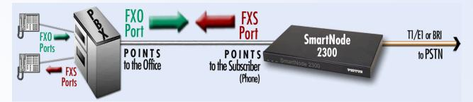
However you can NOT connect a SmartNode 2300 IC-4FXS (FXS) card to the CO (FXS).
