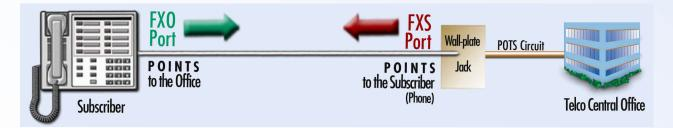
**FXO - Foreign eXchange Office** interface (the plug on the phone) receives POTS service, typically from a Central <u>Office</u> of the Public Switched Telephone Network (PSTN). In other words an FXO interface **points** to the Telco **office**. An FXO interface provides the following primary service to the Telco network device:
