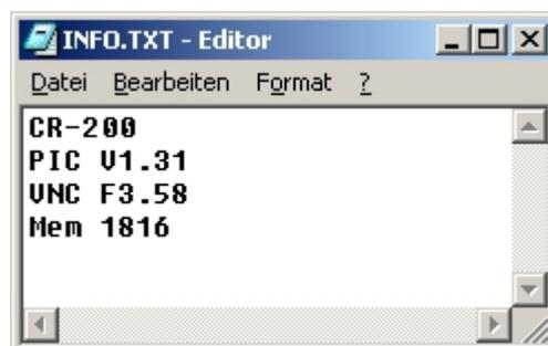
In the first line you see the product name. After that, the software versions of the unit are displayed („PIC“ and „UNC“), which you should report to the support-hotline if asked for. Finally, the free memory space left for recordings on this flashdrive is displayed in minutes („Mem“)..
