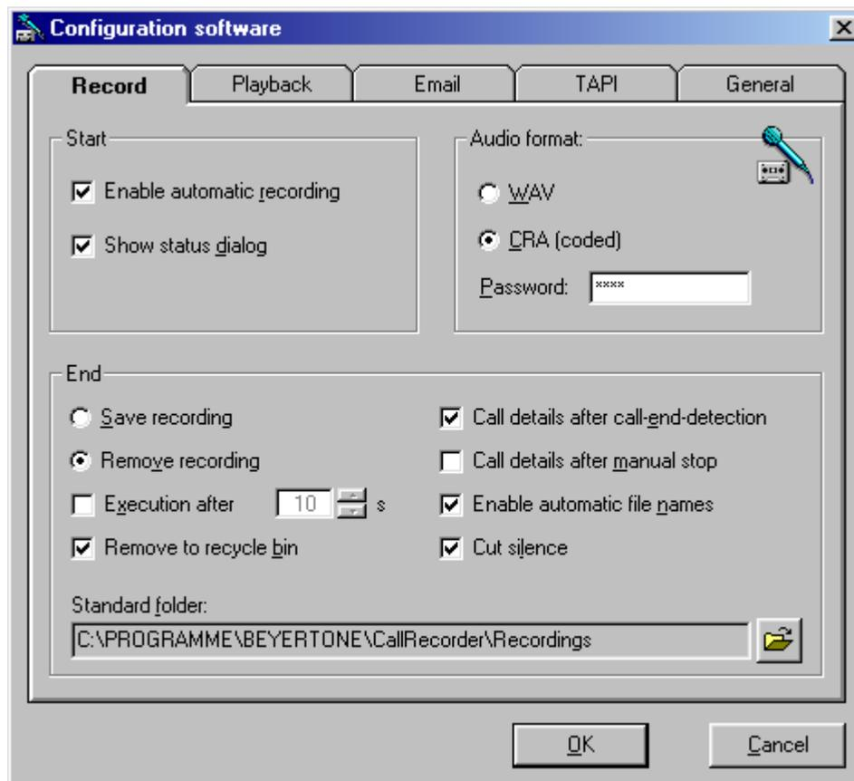
Via 'Enable automatic recording' you cause the software to begin making a recording to file as soon as a start signal is relayed from the CR-100 USB (this can be produced by the press of a button or automatically at the start of every conversation – see section 7.1).
