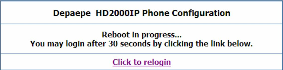
You can reboot the HD2000IP by clicking on the “Reboot” button after each update to the configuration page. Alternatively, you can reboot by unplugging the power supply of the HD2000IP and then powering it on again. If your HD2000IP ever becomes “stuck” or un-responsive, you can unplug the power supply to reboot it. Frequent rebooting by unplugging the power supply is not recommended and should not be necessary.
