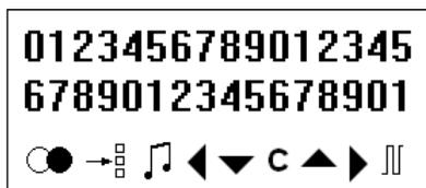
The two uppermost lines display numbers or the menu settings. The lower line displays pictograms that correspond to the functions.
