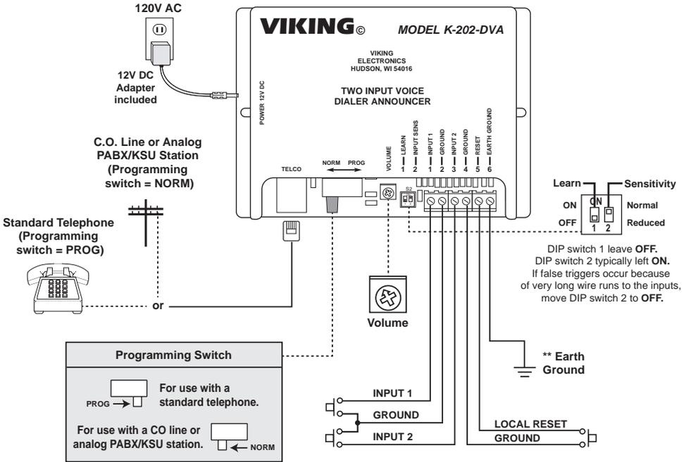
**\*\* Note:** To increase surge protection, fasten a wire from this screw terminal to Earth Ground (grounding rod, water pipe, etc.)
