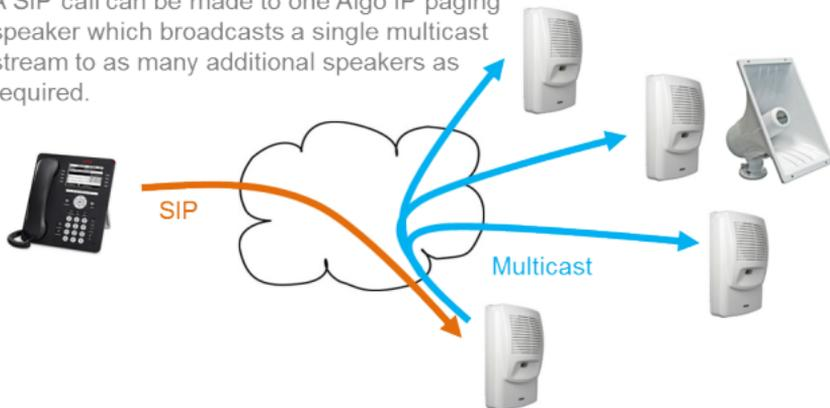
In the diagram above, the bottom 8180 is configured with a SIP Page Extension. When called from a phone, the SIP registered 8180 auto-answers and plays the page audio over its speaker. Simultaneously, the bottom 8180 broadcasts the audio over the network using multicast to as many additional 8180s as required (or 8188 ceiling speakers).
