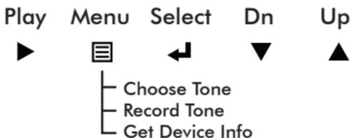
The Program buttons on the back of the 8180 allow local adjustment of alert tones and alert volume. The buttons are intentionally hidden from view after installation and can be disabled using the web interface.
