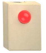
When used with an analog phone line, the **VR-1A** will provide "ring" indication, "on the phone" indication and "message waiting" indication for both "stutter dial tone" and standard message waiting voltage. In this application the **VR-1A** connects directly to tip and ring.
