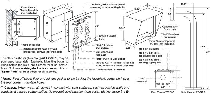
**1600-20A** always bring conduit into the bottom of the unit. If this is not possible, drill a 1/4" (not included) diameter hole in the bottom of the black plastic box.
