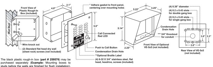
\* **Note:** Peel off paper liner and adhere gasket to the back of the faceplate, centering it over the four corner mounting holes.
