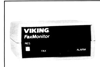
FaxMonitor allows you to "check the fax" without leaving your desk. Since most fax machines are not located next to the desk, the FaxMonitor provides the convenience of a remote "message waiting" indication the minute a fax has arrived. FaxMonitor gives a short, attention-getting tone burst when the fax transmission is complete.
