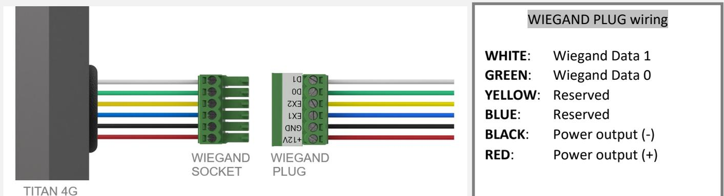
The Wiegand input can accept the following standard formats: 8-bit keystroke, 26-bit, 32-bit, 34-bit codelock and RFID reader.
