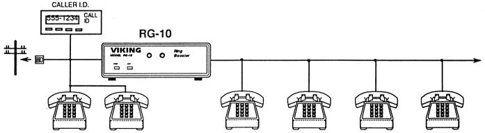
Up to 5 one REN phones (for a typical C.O. Line) may be installed ahead of the RG-10.
