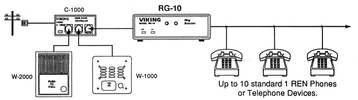
USE WITH CALLER ID: Equipment providing caller ID features must to be installed ahead of the RG-10.
