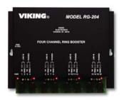
The RG-204 ring generator is designed to reshape and increase the ringing power of up to 4 analog PABX extensions, FXS ports, IP phone system analog ports, or any other telecom devices which provides ringing. The RG-204 duplicates the incoming ring cadence allowing it to be compatible with custom ringing features. For more information on the RG-204, see DOD# 417.
