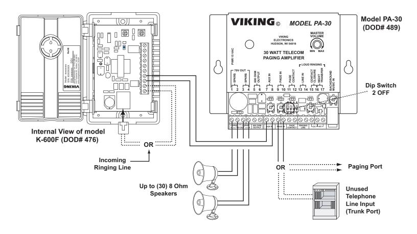
In the Viking model PA-30 amplifier, voice paging is a higher priority than loud ring, meaning loud ring is not heard while a page is in progress. Some customers want loud ring to be a higher priority than a voice page. This is easily accomplished by adding a K-600F to the PA-30, wiring the K-600F to the auxiliary input of the PA-30 and setting PA-30 dip switch 2 to off. Loud ring is now a higher priority than a voice page.
