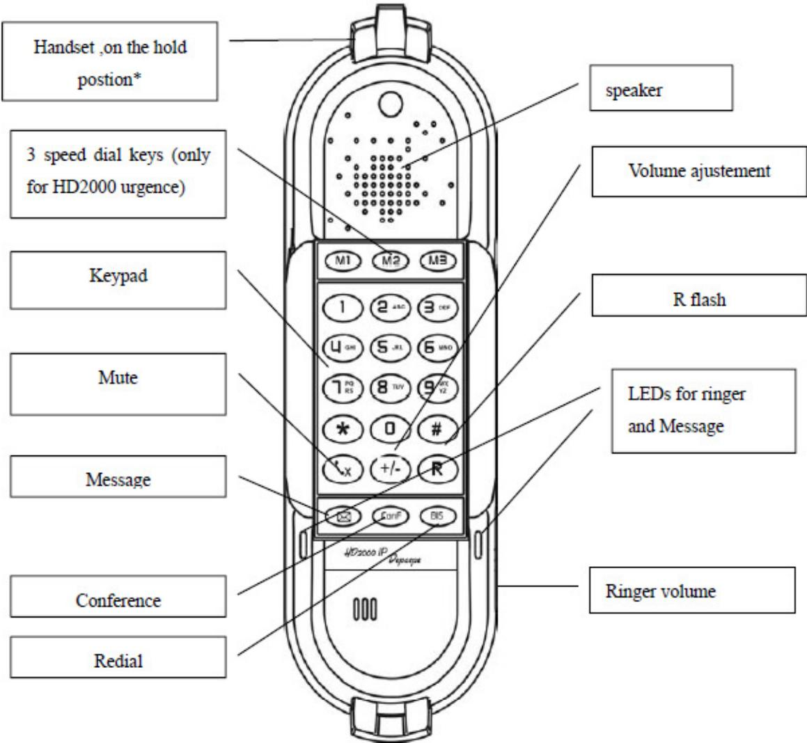
\*Handset on hold position: This feature can be used to secure the handset while waiting for someone to 'come to the phone' without going back to on-hook condition.
