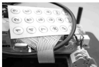
Internal keypad to access to the main IP parameters
